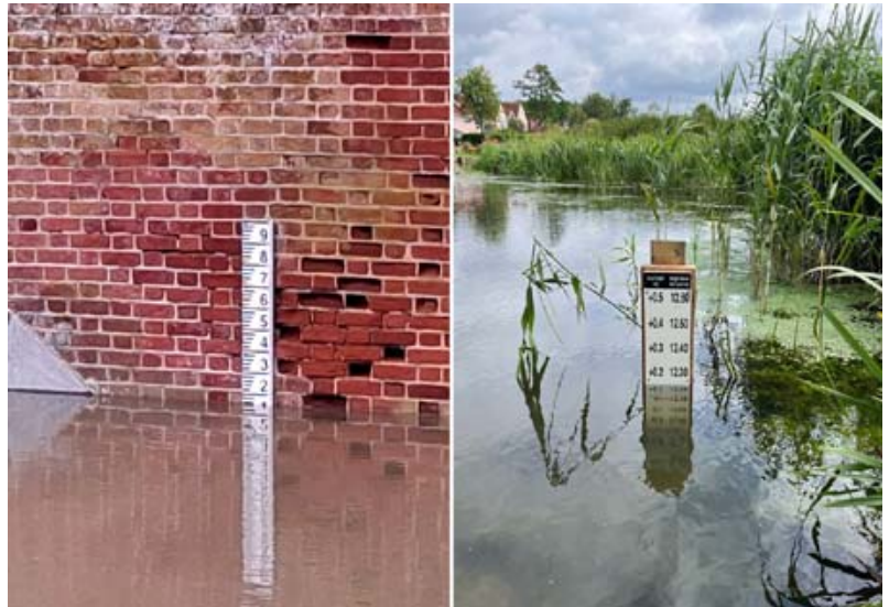
↑ Water level gauges at Abel Bridge and Caley Green show the levels were up by .15m local level. Thanks to Antony Day for these photos taken on 29th January.
